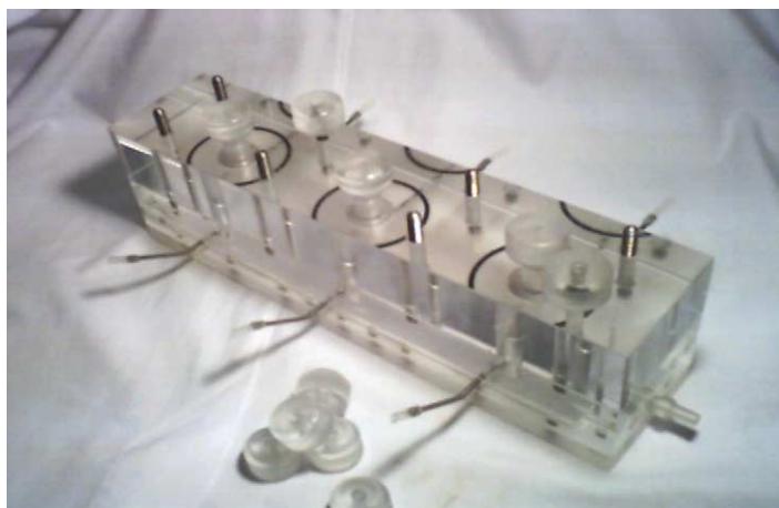
Fig. 2. Diffusion chamber constructed for this study.
